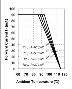
Fig 4. Forward Current Derating Curve
