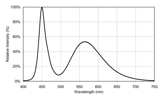
Fig 1. Relative Spectrum of Emission
