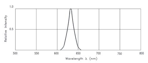
Fig.1 RELATIVE INTENSITY VS. WAVELENGTH
