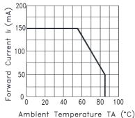
Fig.3 FORWARD CURRENT DERATING CURVE
