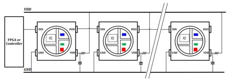
Note: Bypass capacitor is necessary in the design to guarantee good power feed quality and cascade stability.
