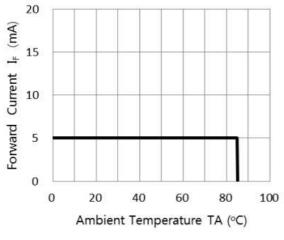
Fig. 2 FORWARD CURRENT VS. DERATING CURVE
