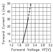
Fig.2 FORWARD CURRENT VS. FORWARD VOLTAGE
