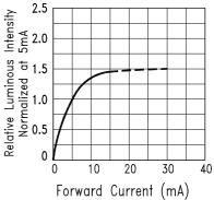
Fig.4 Relative Luminous Intensity
