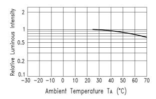
Fig.5 Luminous Intensity vs.
