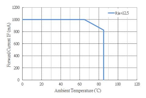
Fig 6. Forward Current Degrading Curve
