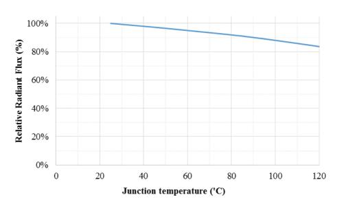
Fig.5 Relative Radiant Flux vs Junction Temperature
