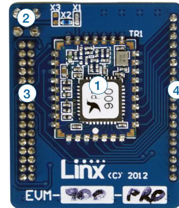
Figure 3: HumPRO™ Series Transceiver Carrier Board
