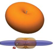
Gain is also related to the overall physical size of the antenna, as well as surrounding materials. As the geometry of the antenna is reduced below the effective wavelength (considered an electrically small antenna) the gain decreases. Also, the relative distance between an electrically small antenna and its associated ground impacts antenna gain.
