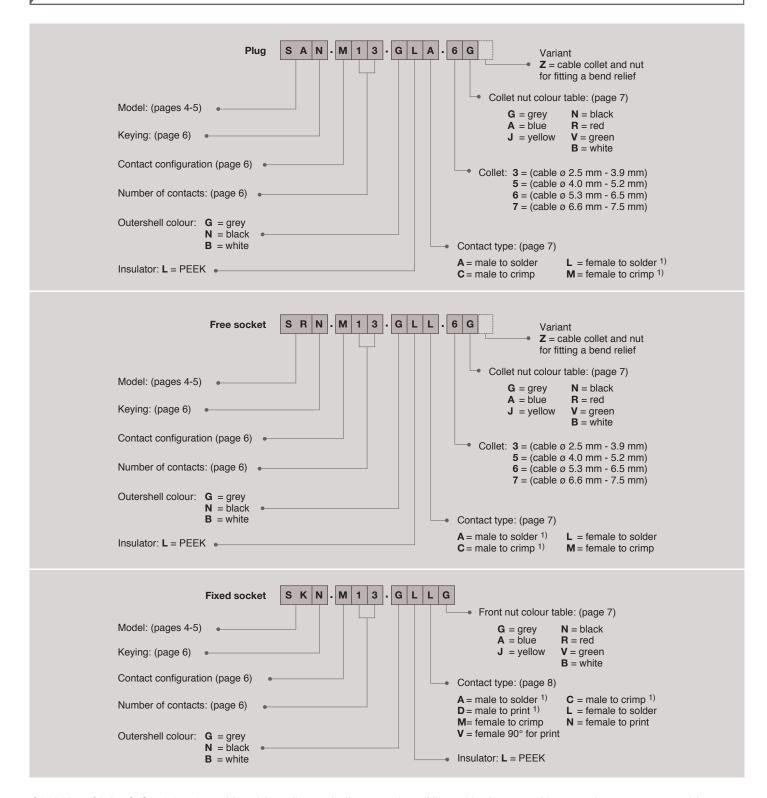
**SAN.M13.GLA.6G** Straight plug with cable collet and alignment key (N), multipole type with 13 male contacts to solder, grey Proprietary sulfone shell, PEEK insulator, collet for max cable  $\emptyset$  6.5 mm and grey collet nut.
