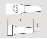
A bend relief absorbs the angular force that may be exerted on cables.
