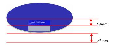
The device case will act as the spacer to keep the antenna from going below the minimum distance.
