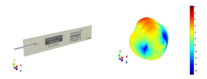
**3D pattern at 890 MHz**Drag to rotate pattern and PCB by using Adobe Reader
