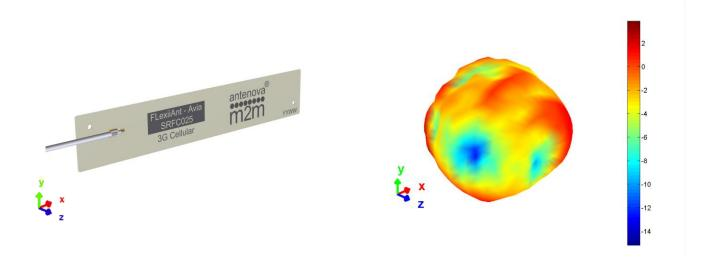
**3D pattern at 1950 MHz**Drag to rotate pattern and PCB by using Adobe Reader
