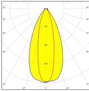
LED Z8Y22T **FWHM** 16.0 + 52.0° Efficiency 90 % Peak intensity 2.5 cd/lm LEDs/each optic
