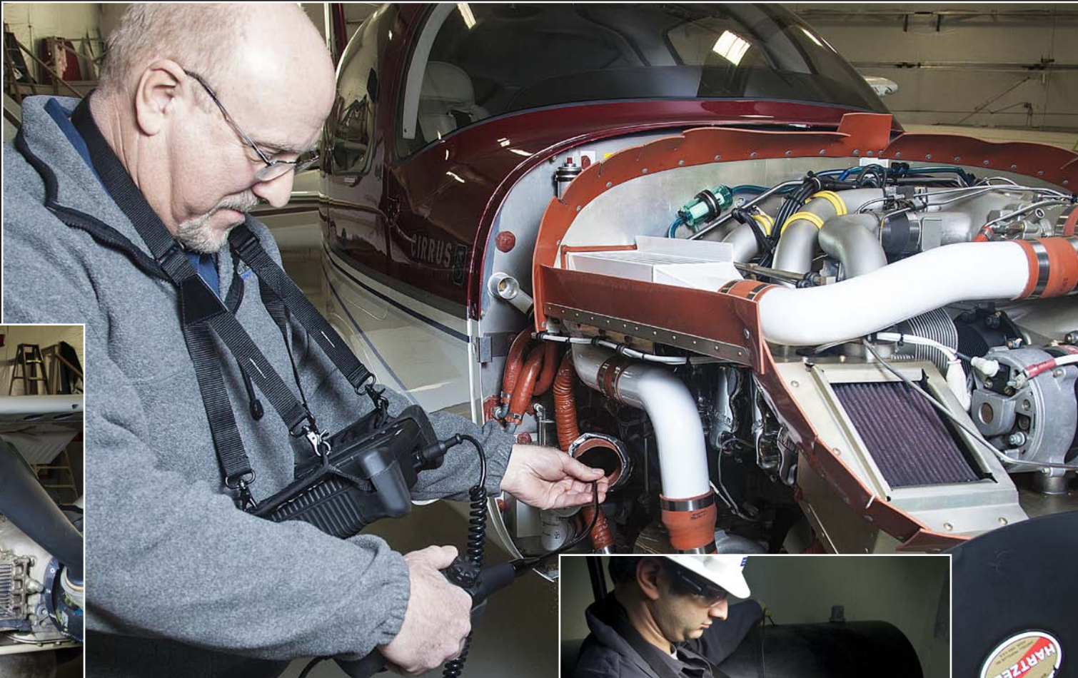
Checking aircraft engines and airframes for cracks, wear, defects and debris; Inspecting oil tank for corrosion
