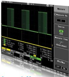
Automatic Measurements Save time making measurements on your signals by using the 26 automatic measurement parameters. See your results color coded to the channels that are being measured. For a more in-depth look turn on the min/max statistics to observe trends in the measurements.
