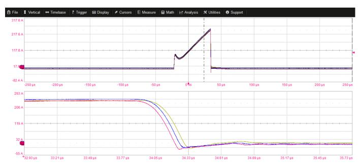
Comparison of three Teledyne Test Tools Rogowski probes. The probes have been offset to enable comparison.
