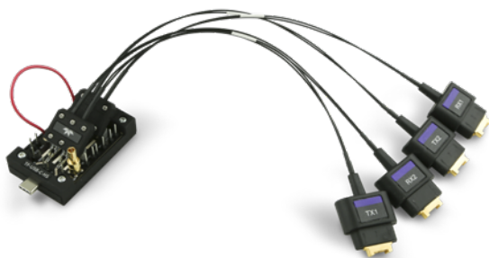
TF-USB-C-HS USB4 High Speed and Sideband Test Coupon
