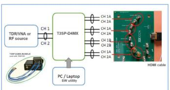
Testing differential impedance for. USB, HDMI, Display Port, Automotive Ethernet ...
