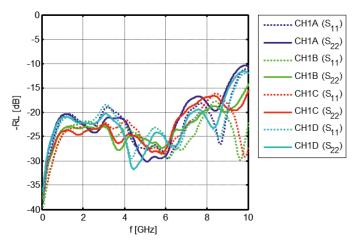
Return loss (RL) of CH1 and CH2-input (S11) when routed to  $50 \Omega$ -terminated output respectively CH1<X> port and CH2<X> port (S22).
