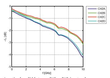
Insertion loss (IL) between CH1 or CH2-input and, respectively, CH1<X> or CH2<X> output ports.
