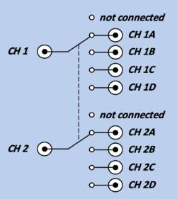
Simplified functional diagram showing input ports CH1 and CH2 to the left and the blocks of four output ports for each input port. Alternatively, the input can be set to an unconnected state.
