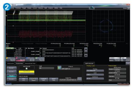
DigRF v4 Constellation diagram shows information such as gaussian noise, Phase noise, and attenuation.
