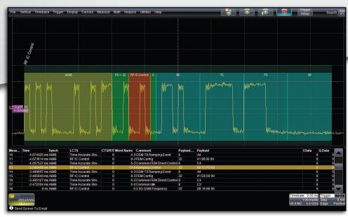
View an entire DigRF 3G burst using intuitive decoding and table display. Click the table to view a zoom of a particular packet.
