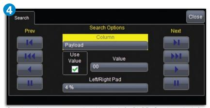
Search can locate up to 14 selectable criteria for DigRF 3G and 18 criteria for DigRF v4, or narrow down the search by entering a value.
