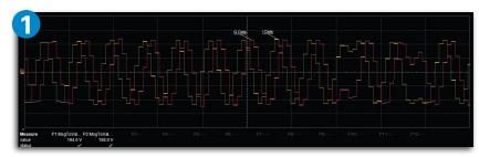
Convert the digital I and Q DigRF 3G signals into corresponding analog waveforms for easy analysis.
