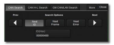
Search through long records of decoded data by entering specific message or frame details.
