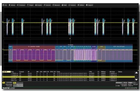
With CAN and CAN FD trigger and decode the oscilloscope becomes the ideal tool for debugging CAN controllers, busses and systems. Identify and isolate specific frames with ID, Remote and Error frame triggering. Decoding CAN signals provides tremendous insight into activity on the bus, and measurement tools enable fast analysis of bus performance.
