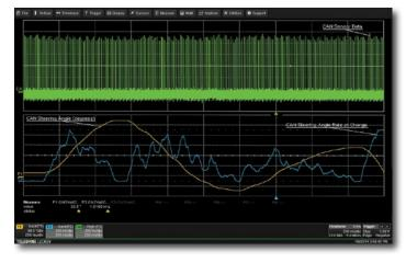
Information on the steering angle and steering angle rate of change is extracted from the CAN message acquisition, rescaled to decimal values, and plotted as a time-correlated "Track"
