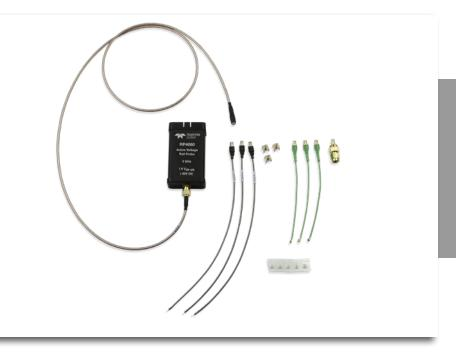
The RP4060 and RP2060 probes are designed specifically to probe low-impedance DC power/voltage rails. Low attenuation means a lownoise view of small signal variations at high frequency, while the probe's built-in offset of up to ±60V enables compensation for the rail's DC voltage. The probe's high DC input impedance eliminates loading of the low-impedance DC rail.
