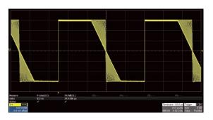
The rise/fall times can be set independently to a minimum of 16.8 ns at any frequency and to a maximum of 22.4s.
