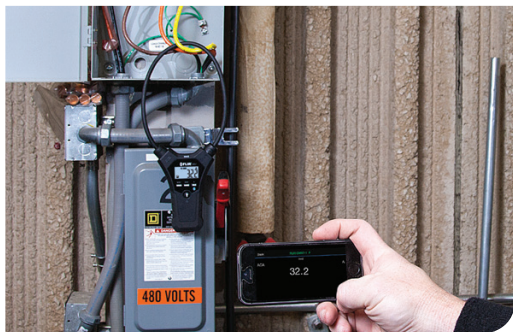
Bluetooth capability gives readings at safe distances
