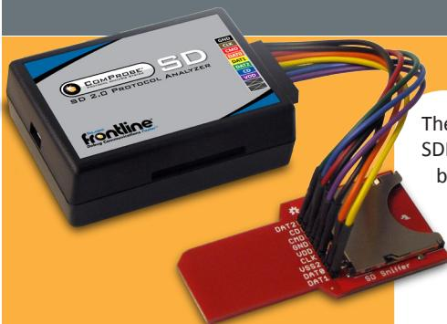
The Frontline SD Protocol Analyzer includes powerful Frontline software and the SD/SDIO/SPI/MMC hardware interface.
