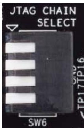
Figure 3. PCI Express Board Configuration/Programming Mux Selection
