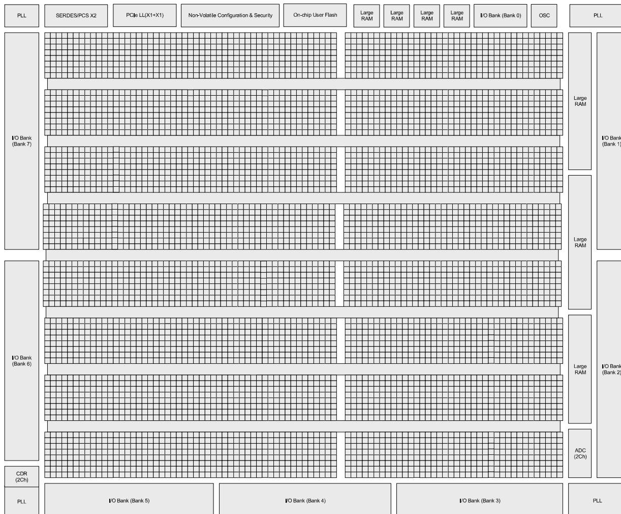
Figure 2.2. Simplified Block Diagram, MachXO5-NX-55T Device (Top Level)
