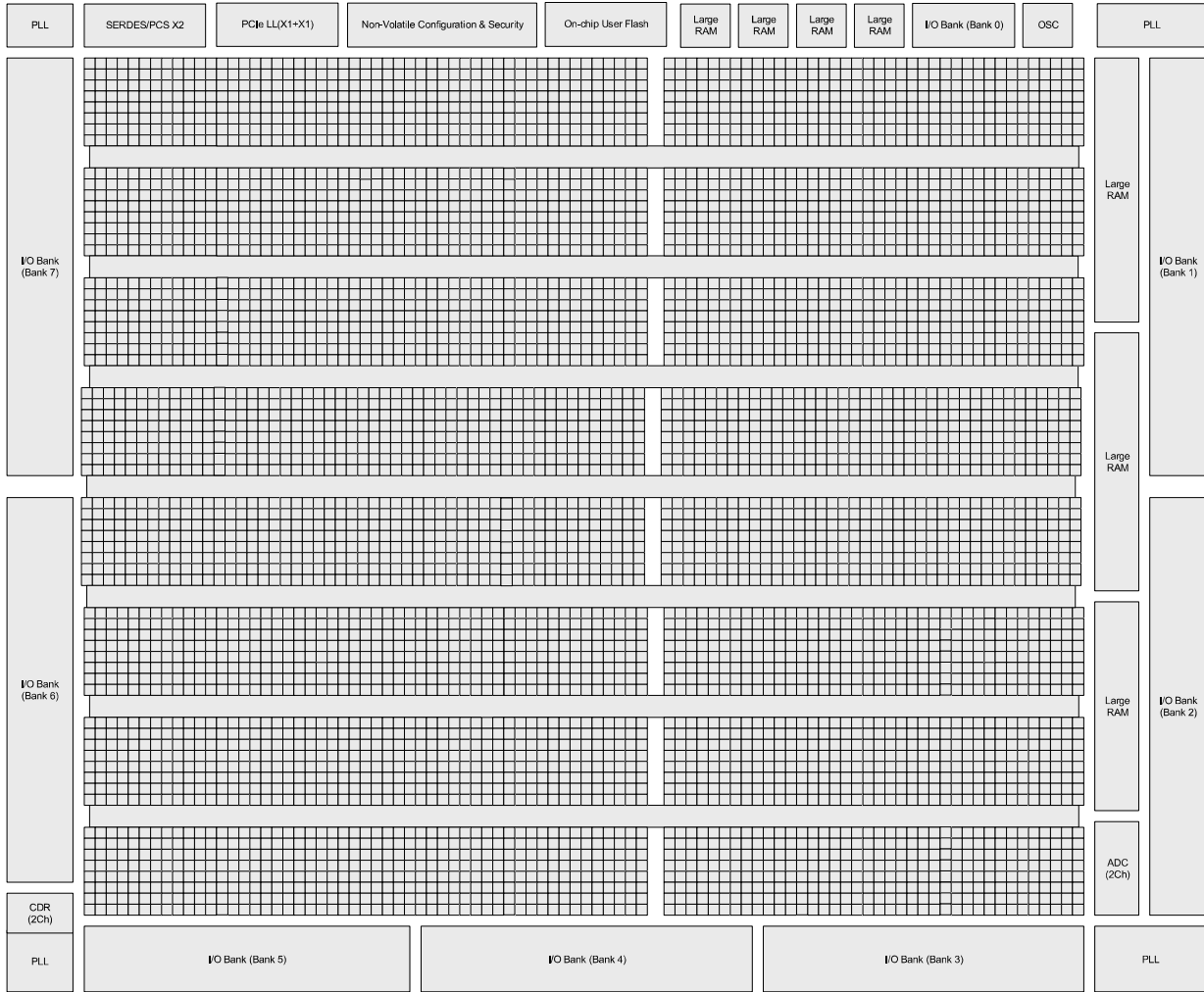
Figure 2.3. Simplified Block Diagram, MachXO5-NX-100T Device (Top Level)
