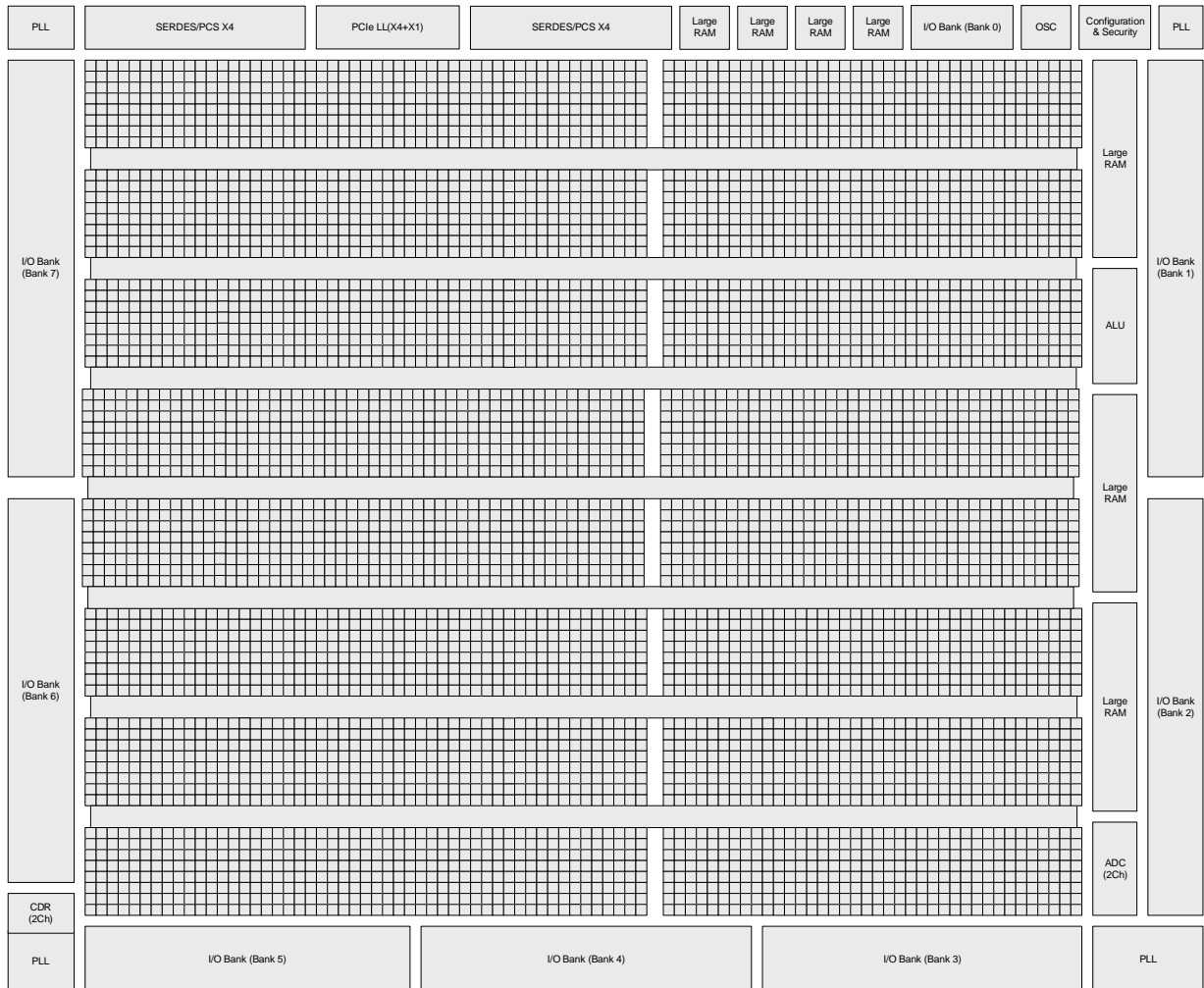
Figure 2.2. Simplified Block Diagram, LFCPNX-100 Device (Top Level)
