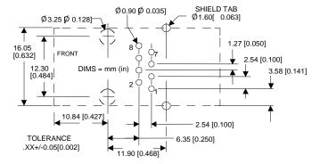
For proper heat dissipation, the PCB should have approximately 1 square inch of copper attached to the shield tabs. The shield tabs are an important source of heat sinking for the device.
