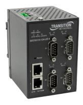
Transition Networks serial device server provides the ability to communicate serial data across an Ethernet network. The SDSTX3110-124-LRT-B contains (2) 10/100Base Fast Ethernet ports that can be configured to one or multiple redundant servers. Security of the data transmission is assured through HTTPS, SSH, and SSL data encryption.
