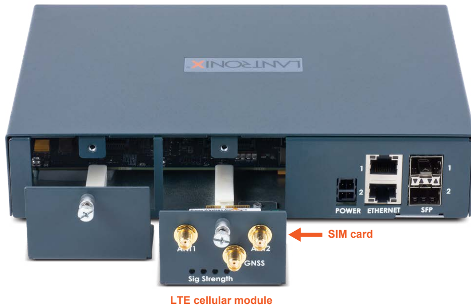
Figure 2-13 EMG 8500 LTE Cellular Modem Module
