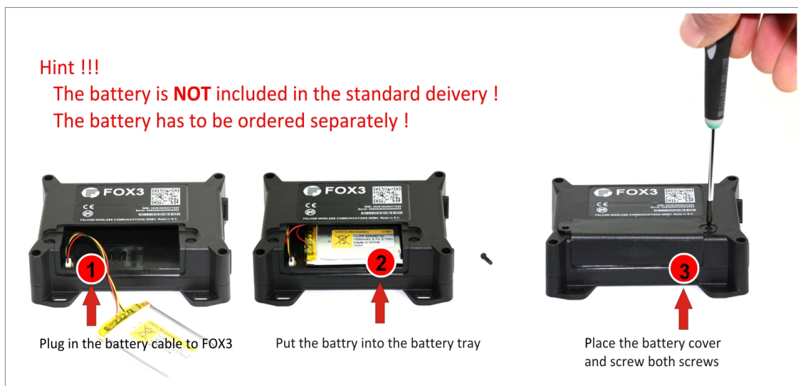
Figure 14.1: Connecting the battery to the FOX3-2G/3G/4G devices
