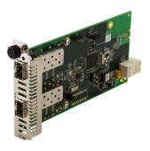
The ION C3100 is a fiber to fiber media converter module. It is protocol independent and supports data rates from 100Mbps to 2.5Gbps through two open SFP slots. This any-rate to same-rate converter can be used to perform reliable and cost-effective single mode to multimode fiber conversion or it can be used to provide wavelength conversion in CWDM applications. The ION C3100 is a manageable device when installed in a managed ION chassis.
