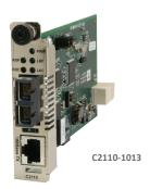
The ION C2110 is a media converter module that provides an interface between 100Base-TX ports and 100Base-FX ports, allowing users to integrate fiber optic cabling into 100Base-TX copper environments. Operating at Layer 1, the physical layer, data is passed through the converter at line speed, making it ideal for applications where low latency is essential. The ION C2110 is a manageable device when installed in a managed ION chassis.
