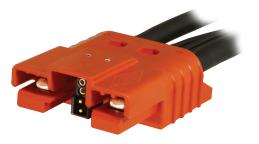
SBE<sup>°</sup> and SBO<sup>°</sup> connectors build on the capability of the two pole SB<sup>°</sup> connectors by offering up to 8 auxiliary power / signal contacts along with an IEC 60950 touch safe housing. The center of the main connector features a connector holder for either: two PP15/45, two PPMX, or APP's innovative 1x4 auxiliary connector.
