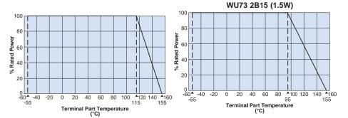
For resistors operated at a terminal part temperature of described for each size or above, the power rating shall be derated in accordance with the derating curve. Please refer to the "Introduction of the derating curves based on terminal part temperature" in the beginning of the catalog.
