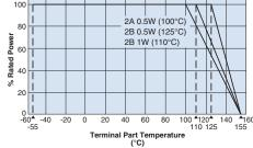
For resistors operated at a terminal part temperature of described for each size or above, the power rating shall be derated in accordance with the above derating curve. Please refer to "Introduction of the derating curve based on the terminal part temperature" in the beginning of our catalog prior use.
