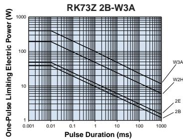
Please ask us about the resistance characteristic of continuous applied pulse. Please calculate One-Pulse Limiting Electric Power using upper limit of resistance (50mΩ or 100mΩ) for applied current. The pulse endurance values are not assured values, so be sure to check the products on actual equipment when you use them.
