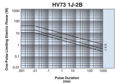
The maximum applicable voltage is equal to the max. overload voltage. Please contact factory for resistance characteristics of continuous applied pulse.
