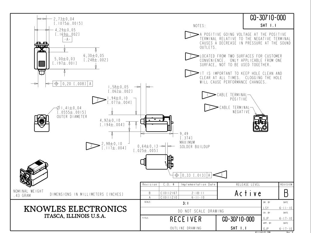
UNDAMPED MAGNETIC BALANCED ARMATURE RECEIVERS INTENDED FOR USE AS THE HIGH AND LOW FREQUENCY DRIVERS IN A HI FI SYSTEM. THE GQ RECEIVER COMBINES A WBFK AND ED RECEIVERS COUPLED THROUGH A CIRCUIT TO PROVIDE THE RESPONSE SHAPE.
