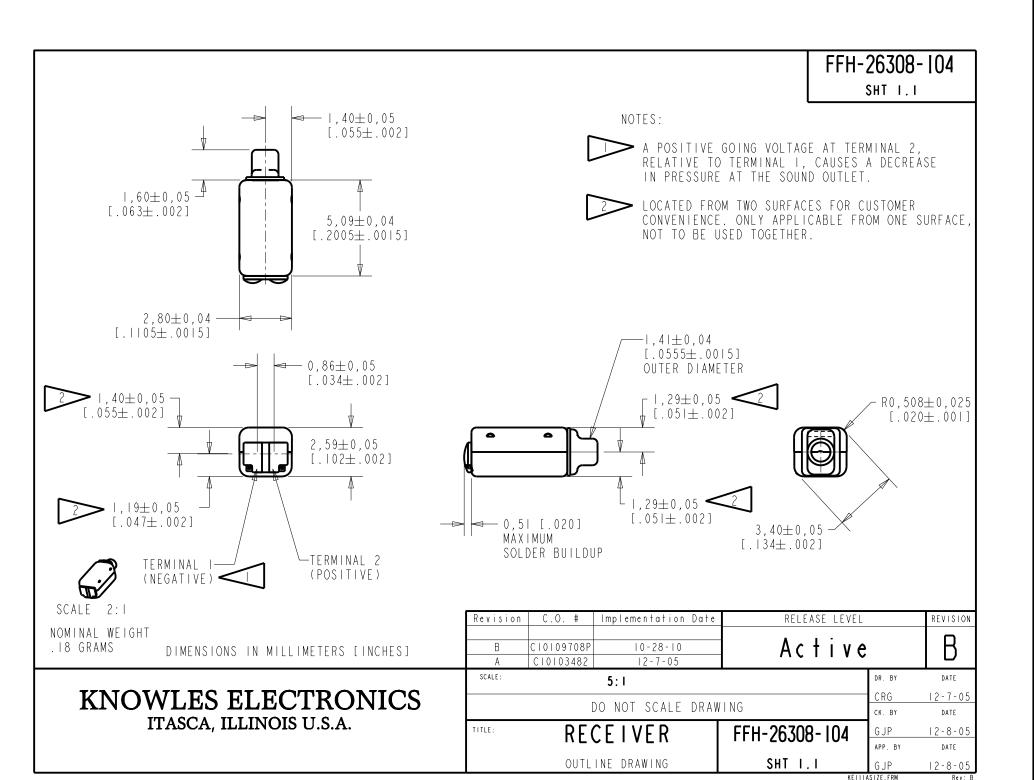
THE FFH-26308-104 IS A FERROFLUID AND TYPE III DAMPED FH-26308 RECEIVER WITH A PEAK OF 4dB RELATIVE TO THE SENSITIVITY AT IKHZ UNDER CONSTANT VOLTAGE DRIVE CONDITIONS.
