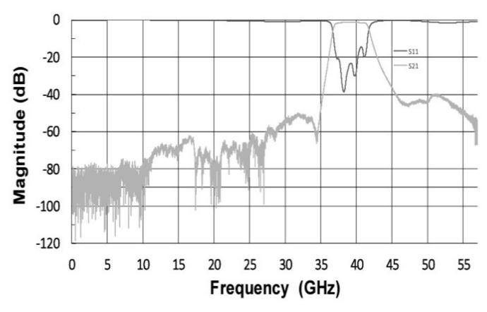
\*Typical de-embedded measured performance mounted on a connectorized test fixture. DEB is 0.010in RO4350B with 50.00hm CPW ground traces going into the ports at room temperature.
