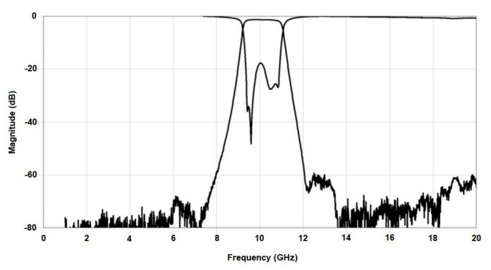
\*Typical de-embedded measured performance mounted on a connectorized test fixture. DEB is 0.010in RO4350B with 50.00hm CPW ground traces going into the ports at room temperature.
