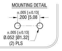
THIS DOCUMENT IS THE PROPERTY OF KEYSTONE ELECTRONICS CORP. AND SHALL NOT BE REPRODUCED, DISTRIBUTED OR USED AS A BASIS FOR MANUFACTURE WITHOUT PROP WRITTEN PERMISSION FROM KEYSTONE ELECTRONICS CORP.
