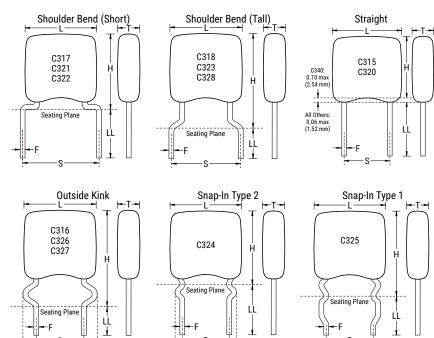
\* May be supplied in a "Shoulder Bend" or "Straight" Lead configuration. Please see Capacitance Range Waterfall section of this document to determine lead configuration availability by capacitance value.
