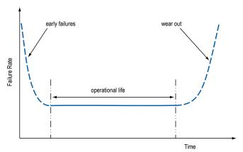
The failure rate is derived from our periodic test results. The failure rate ( $\lambda_R$ ) is, therefore, only given at test temperature for life tests. An estimation is also given at 60°C. The expected failure rate for this capacitor range is based on our periodic test results for capacitors with structural similarity.
