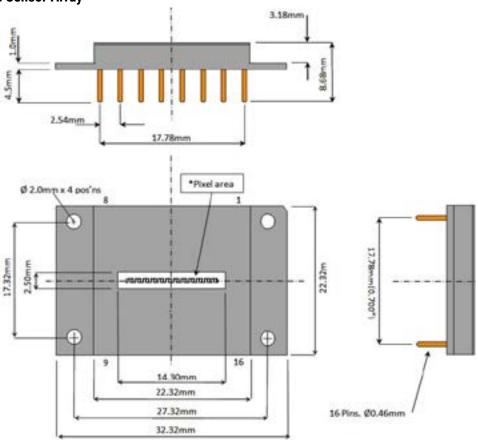
Pin Configuration of Sensor - 510 Element Line Sensor Array
