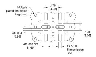
Dimensions are in Inches [Millimeters] 1P520S Mounting Footprint
