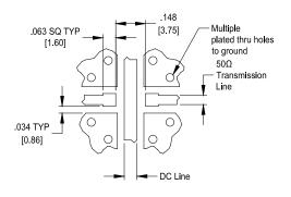
Dimensions are in Inches [Millimeters] X2AS Rev A Mounting Footprint
