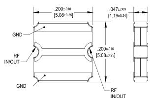
Dimensions are in Inches [Millimeters] X2AS Mechanical Outline
