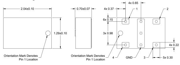
Dimensions are in Millimeters
